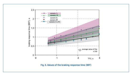
As shown by Jurecki et al. [13], the average values of the response time for both variants of scenario 2, i.e. 2L and 2R, can be considered equal. Figure 5 also illustrates the range of the driver response time determined for the average value of the +/- standard deviation for each analysed scenario.
