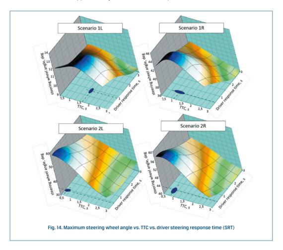
From the diagrams in Figs. 13 and 14 it is evident that the steering responses were more intensive and more varied than the braking responses. It should also be noted that the steering responses were more dependent on the test scenario.
