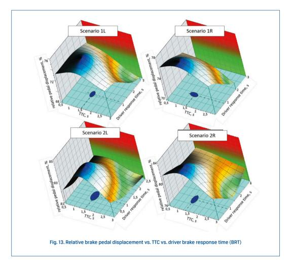
From the diagrams it is clear that the maximum values of the brake pedal displacement were reported at similar values of the TTC and the response time for all the drivers in all the scenarios. In all the scenarios considered, the test runs during which the intensity of the braking manoeuvre was the highest were those with the time-to-collision ranging from 1.2 s to 2.0 s (like in Fig. 11 showing the average values). The highest values were recorded at a TTC of about 1.5 s.
