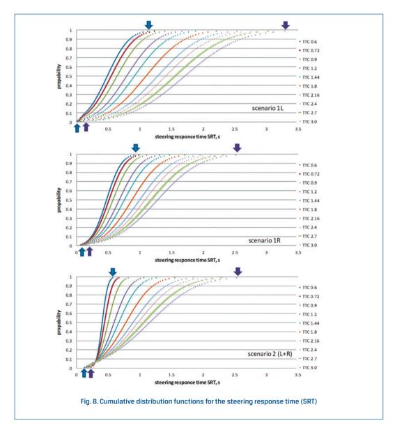
the moment at which a particular response is initiated. It was thus vital to thoroughly analyse the curves plotted for the particular driver responses (braking and steering).
