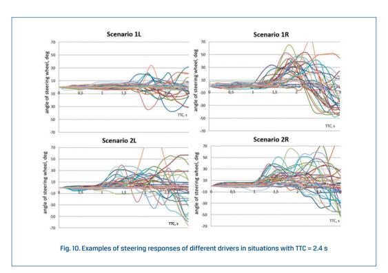
the braking manoeuvre (brake pedal displacement) and the steering manoeuvre (steering angle), for each of the 30 drivers used in each of the test runs conducted.
